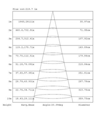
Luminous Intensity Distribution Diagram - At 3000K:
