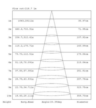
Luminous Intensity Distribution Diagram - At 3000K:
