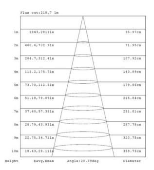
Luminous Intensity Distribution Diagram - At 3000K:
