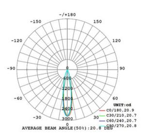
Luminous Intensity Distribution Diagram - At 3000K:
