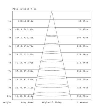
Luminous Intensity Distribution Diagram - At 3000K:
