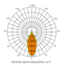
Lumens: 3454.8 Lm UNIT: cd Watts: 40 W – C0/180,23.6,23.1 LPW: 86.37 Lm/W – C90/270,23.2,24.0 CCT: 3000K
