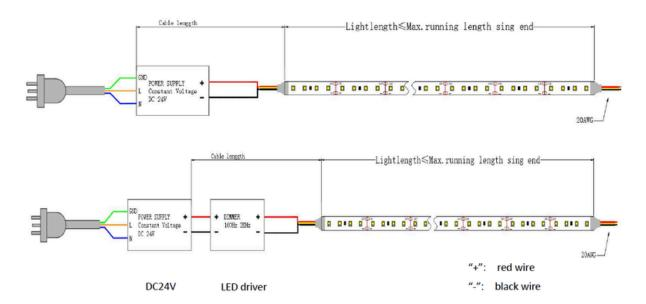
( PS : Strip positive connect to the driver positive, Strip negative connect to driver negative )
