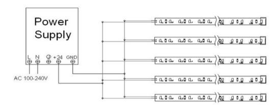
The max running length for each line is 3 meters. Please install the strips in parallel when length is more than 3 meters.
