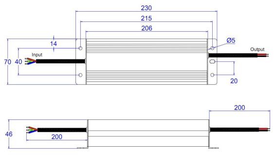
\* Input black(L) and white(N) wires to be connected AC, Green wire to be connected ground; output red and black wires to be connected led lighting.
